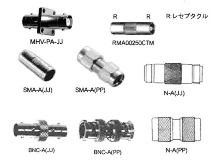
◆The symbol (P),(J) used as connector names for BNC etc is that J means a jack which typically used to mount on panels P means a plug which typically used to attach to co-axial cable.
